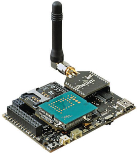
Lowering power requirements for sensor networks is as important as finding new sources of energy. The open-source Wasp mote wireless sensor network platform from Libelium consumes only 0.07 \mu A in hibernation mode. Image courtesy of Libelium.
