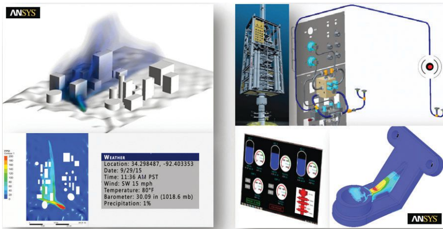
An example of how GE Predix and ANSYS can work together in assessing the environmental, health and safety impact of a plume dispersion from a potential gas pipeline rupture (left); detecting anomalies (top right) and realizing the digital twin of a blowout preventer (bottom right). It's virtual diagnostics/root cause analysis and prognostics/lifting. Images courtesy of ANSYS.
