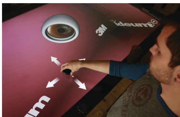
A 3D-printed joystick, made from Graphene 3D Lab's conductive filament, provides a capacitive connection to an interactive smart-table display. Image courtesy of Graphene 3D Lab.
