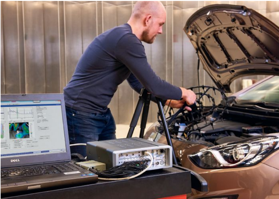
The new High Definition Acoustic Camera can help engineers pinpoint hotspots for NVH generation. Image courtesy of Siemens PLM Software.
