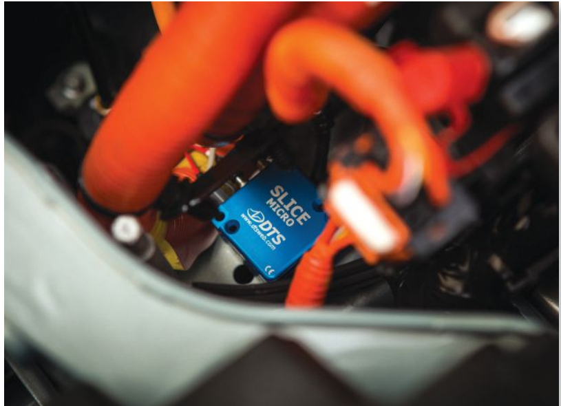
SLICE standalone data acquisition systems are designed for embedded applications with challenging space limitations and rugged test environments. Image courtesy of DTS.
