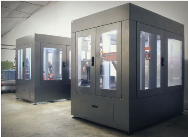
Medium Area Additive Manufacturing (MAAM) filament-based system from Cosine Additive is pictured. The company is particularly targeting the molding and forming market with this system that runs high-fiber-content composite materials. Image courtesy of Cosine Additive.
